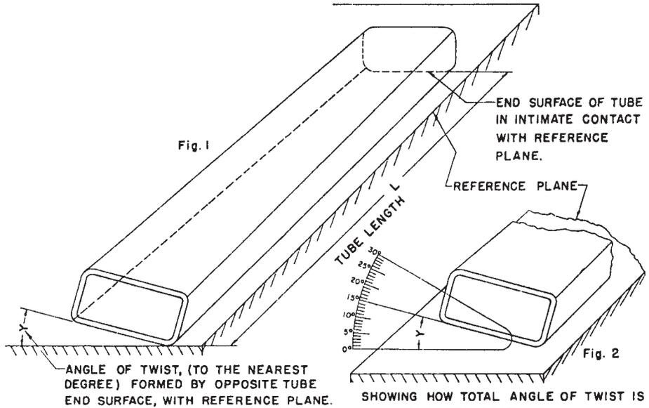
SHOWING HOW TOTAL ANGLE OF TWIST IS MEASURED WITH PROTRACTOR SEGMENT. ANGULAR LINE GOINCIDING WITH TUBE END SURFACE (15° IN THIS ILLUSTRATION) IS THE TOTAL ANGLE OF TWIST.
